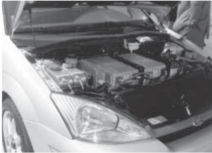
*Under the hood of a hydrogen fuel cell engine.*
