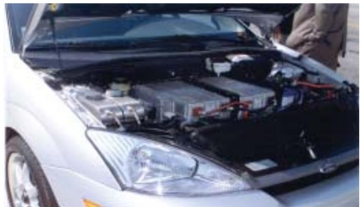
*Under the hood of a fuel-cell powered auto.*
